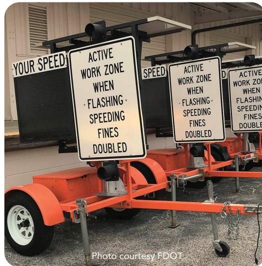
AWAD installed on portable trailers ready for deployment to work zones.
