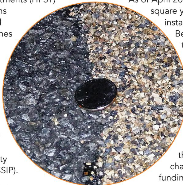
Side-by-side comparison of newly-installed HFST (right) next to traditional surfacing (left).
