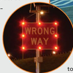
(Left) A rectangular-rapid flashing beacon at night alerts wrong-way drivers of their mistake. (Right) Enhanced pavement markings and signage provide clearer indication to motorists about which lanes lead to Interstate 10 eastbound.
